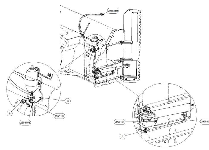
A: The bracket for the cylinder must be installed as in the illustration.
